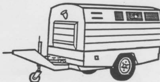
Fig 2. Sound reduced air compressor. The air cooling system is designed to enable the compressor to operate with the canopy fully closed on all sides. The canopy and the chassis are lined with sound absorbent material.
